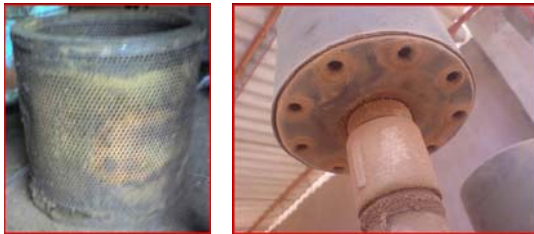
Figure 7 & 8: Choked filters of compressors
